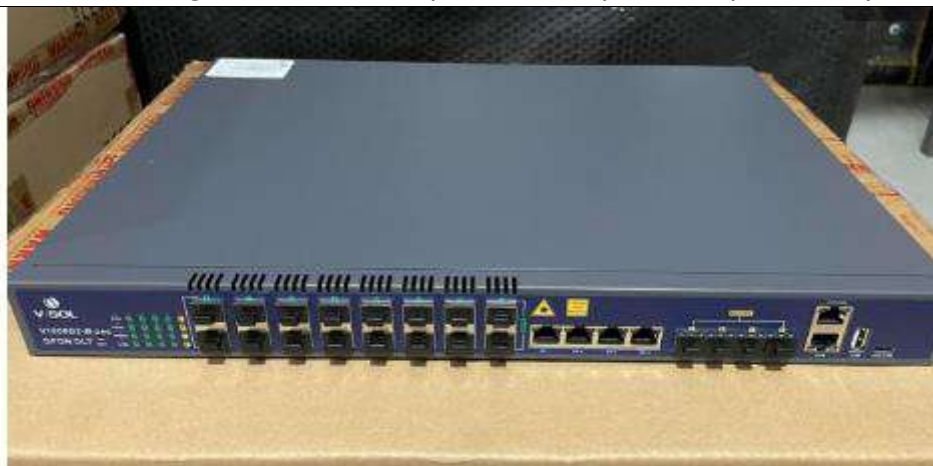
16 PORT GPON OLT (DUAL AC WITH C++++ 9DBM)
